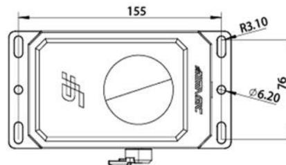
Hole Spacing Layout (mm)
