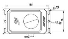
Hole Spacing Layout (mm)
